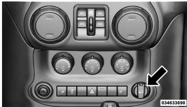
Front Power Outlet
