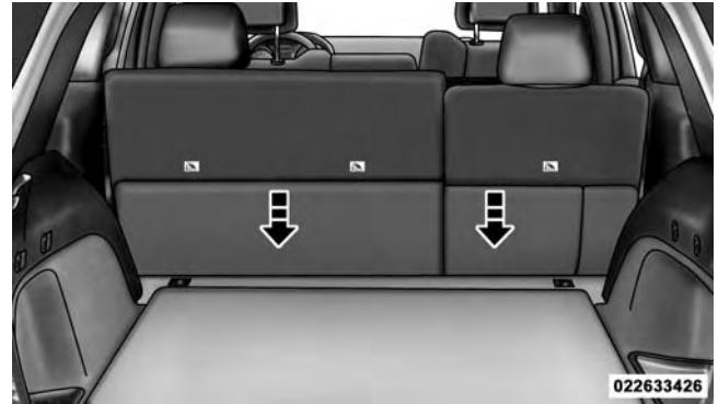
Pulling Down The Carpet Floor Panel To Access Top Tether Strap Anchorage
