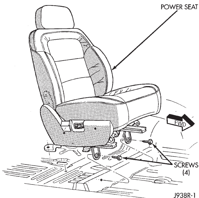
Fig. 4 Power Seat Remove/Install - Typical
